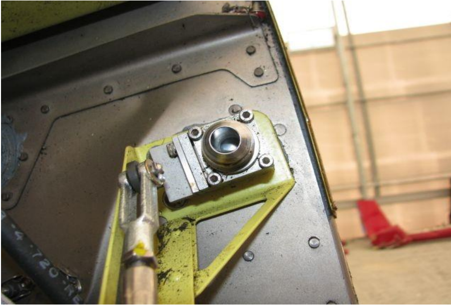
Photo 38 Emergency fuel shutoff valve was found in Off position
