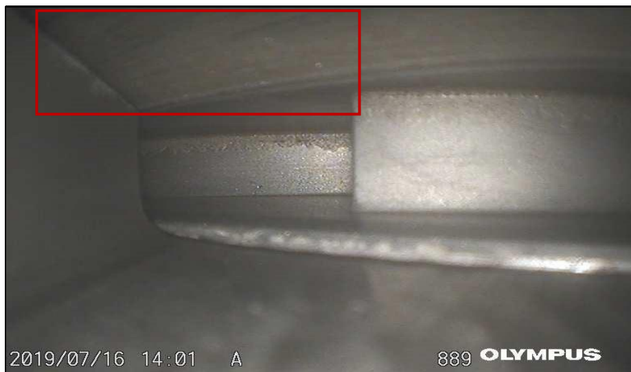
Picture 13 : light rub of compressor cover, at impeller trailing edge (red rectangle).
