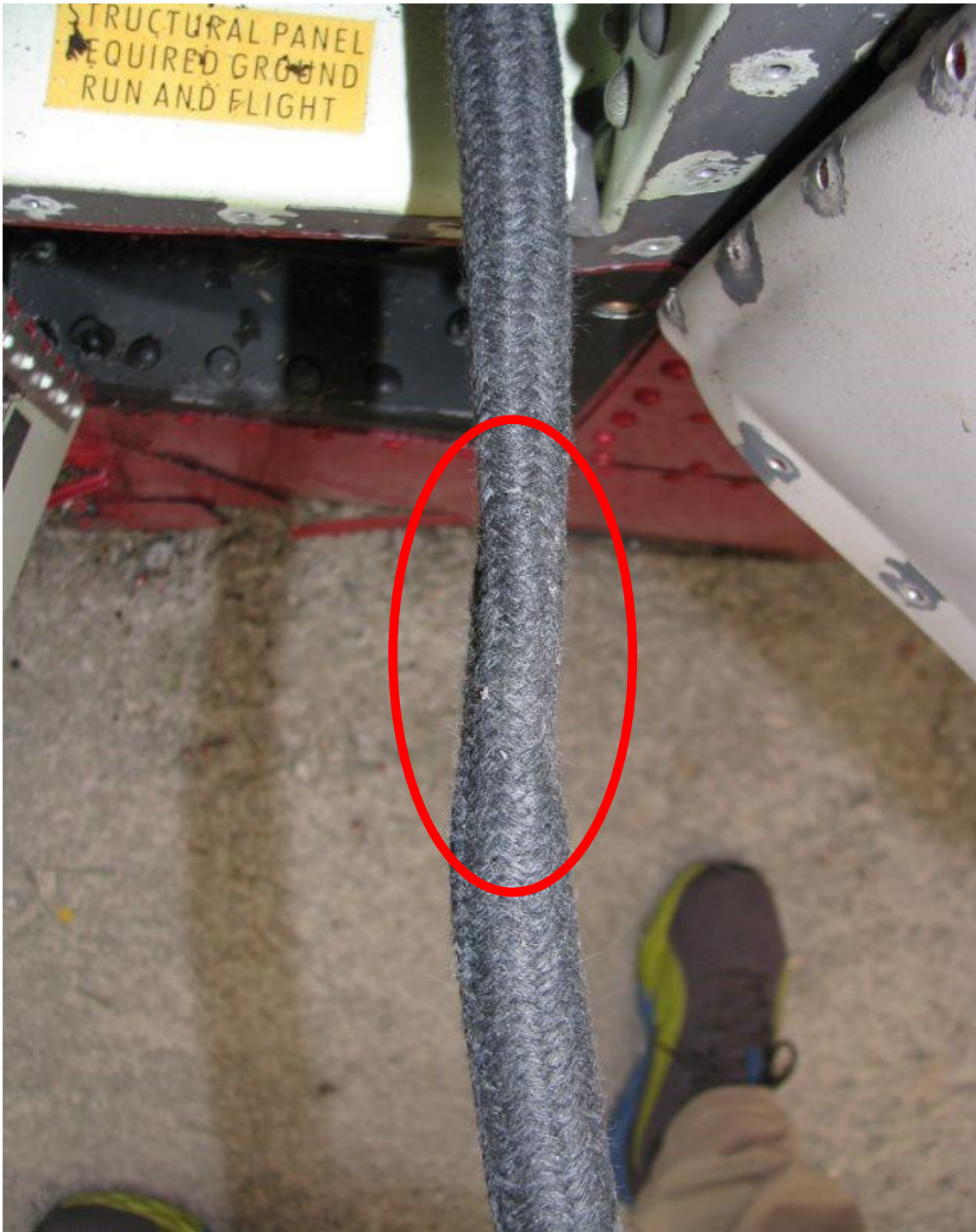
Photo 40 When fuel line was removed, crimped section was observed at area of 90° turn
