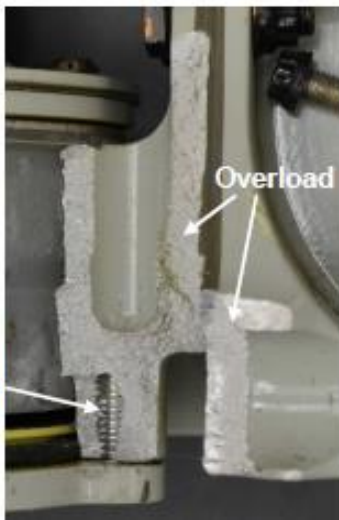
Stud fell out during sectioning
