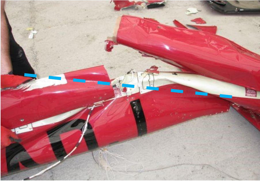
Photo 29 Linear strike mark on left side of tailboom consistent with main rotor strike
