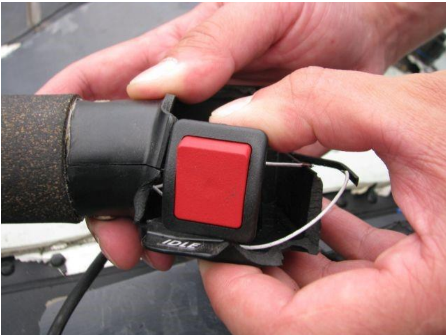
Photo 4 Fly/Idle throttle switch (fractured, but held in place) on collective head was found in Idle position
