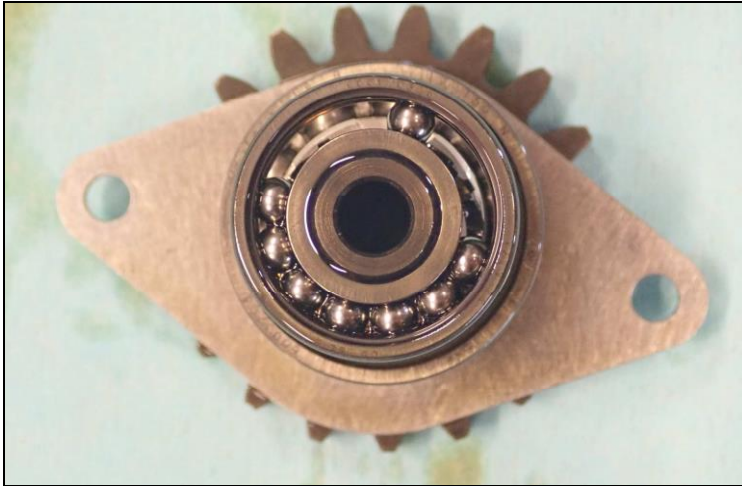
Picture 30 : the front bearing of the HMU's intermediate gear : no ball was missing.
