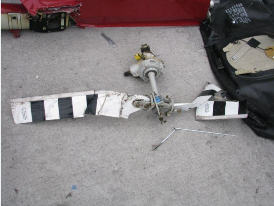
Photo 16 Both blades exhibited impact damage
