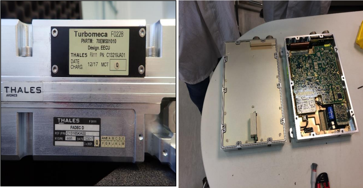
Picture 3 : EECU reference and part number. Thales sealing is unsealed since the examination at BEA.
