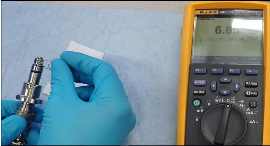
Picture 10 : deliberate contact between two heads of EMP of Module M01 - still with tabs on.
