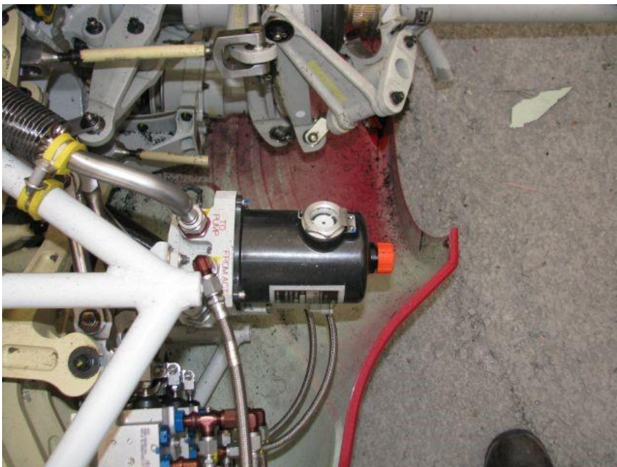
Photo 6 Red colored fluid found on cowling was consistent with hydraulic fluid. Hydraulic reservoir intact.
