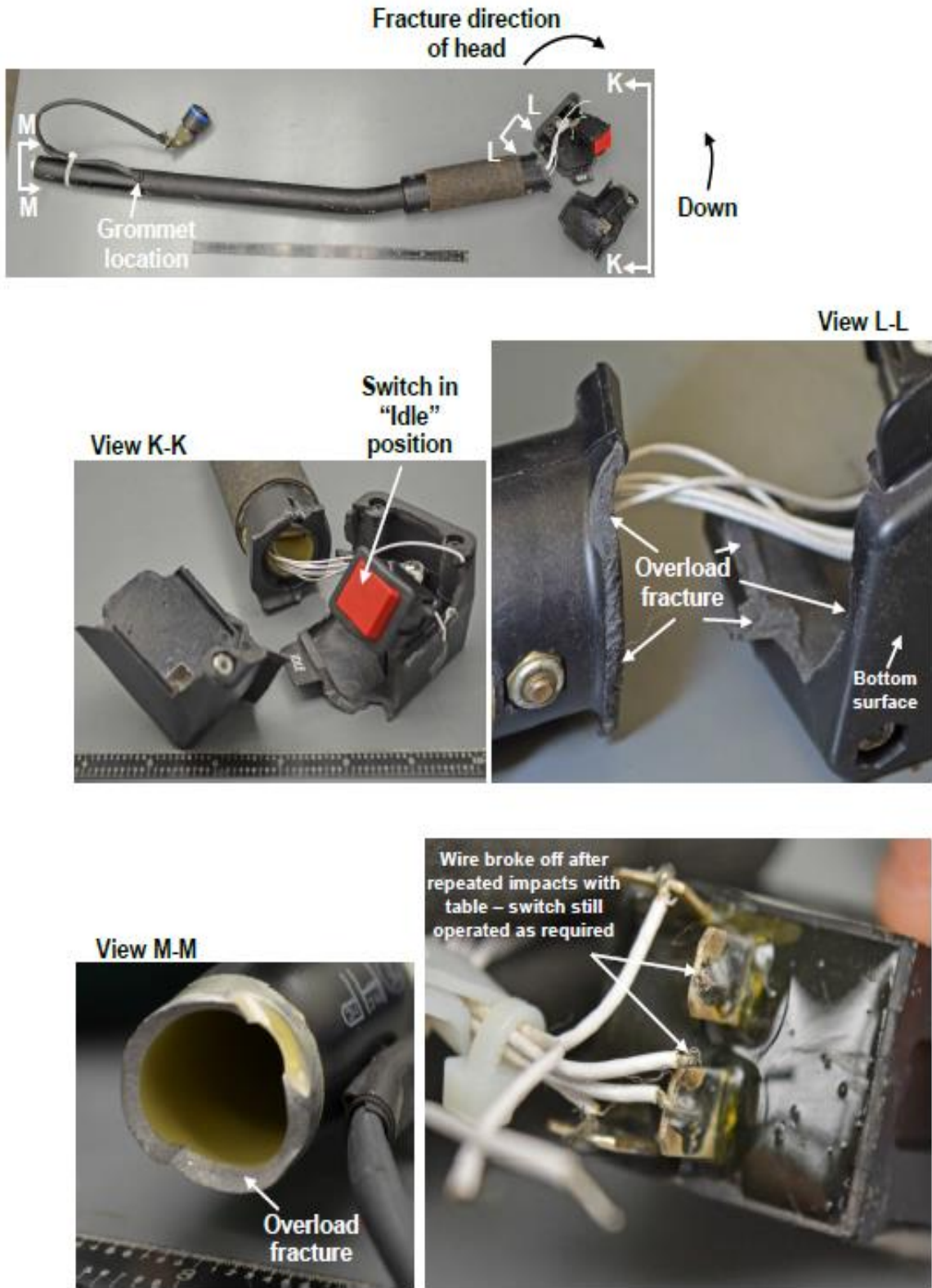
Figure 11: Views of the pilot's collective stick. The fly/idle switch operated as required, even after a wire fractured from a terminal after hitting the switch against the table in the lab.
