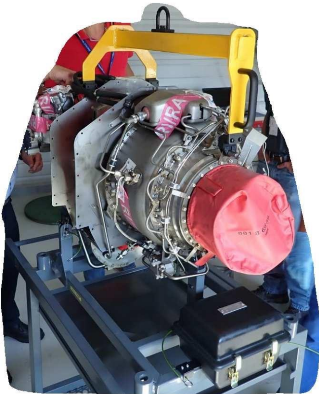
Picture 4 : engine is set on a workshop frame.
