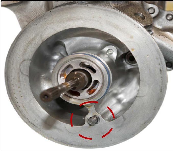
Picture 18 : positioning pin of the HMU below the centering bore and its rubber seal.
