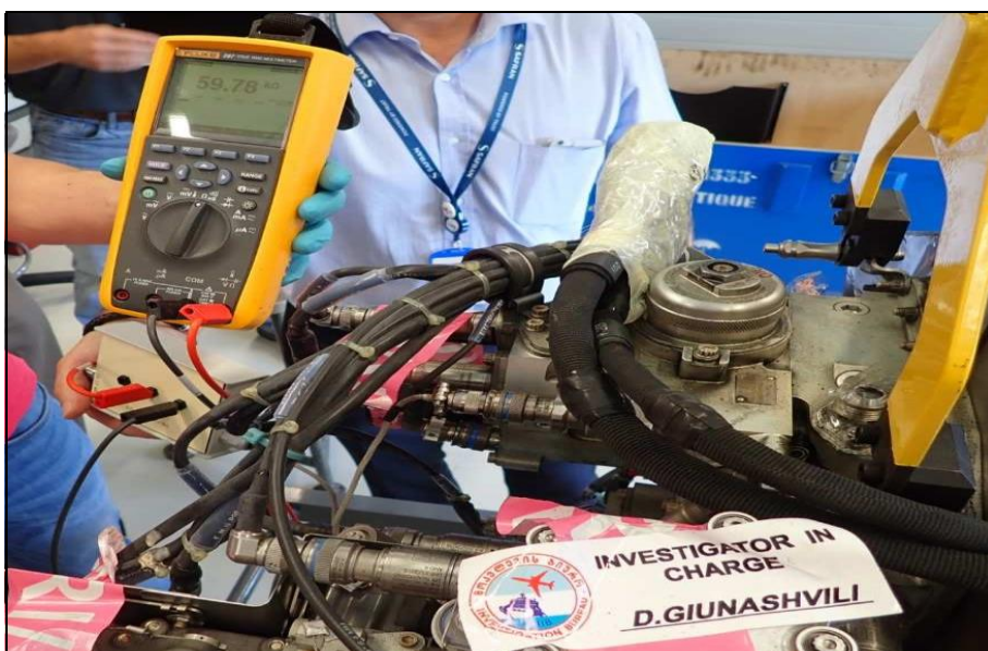
Picture 5 : direct measurement of EMP Module 01 resistance through connector.
