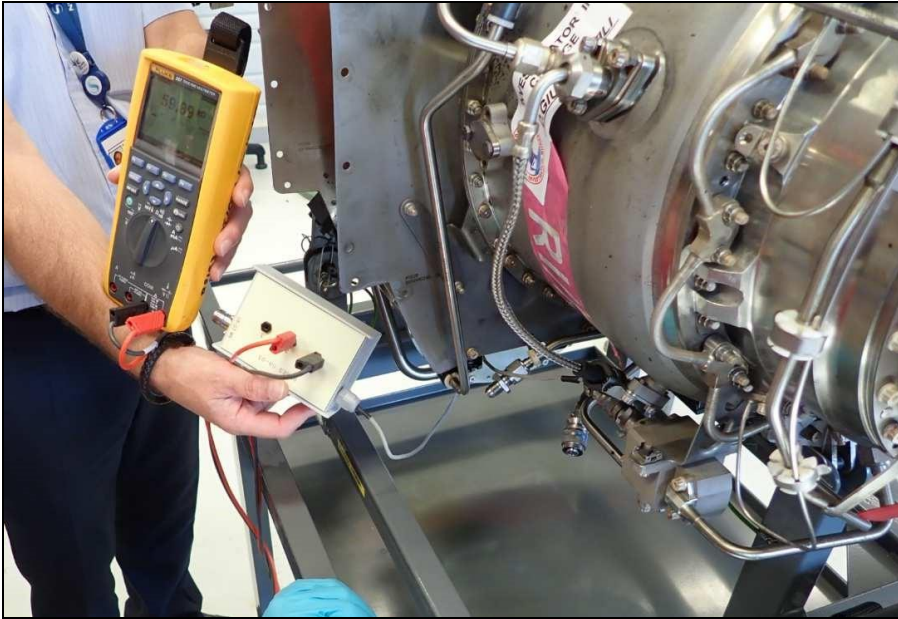
Picture 6 : direct measurement of EMP module M02 resistance through connector.
