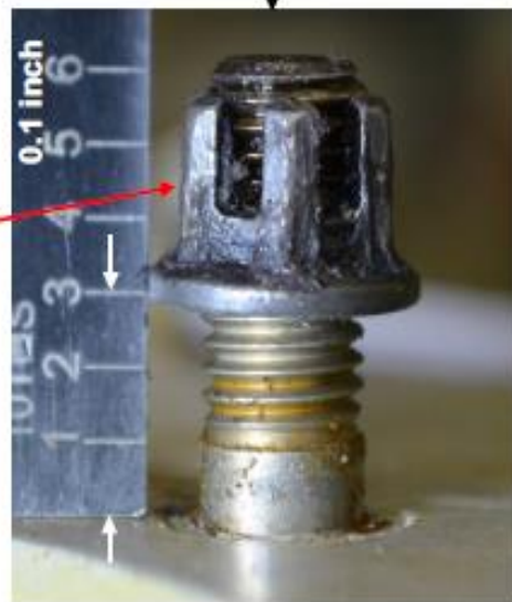
Figure 7: Top photo shows the left-hand LIVE mount assembly. The adapter bridge studs, nuts and safety wire were all intact.
