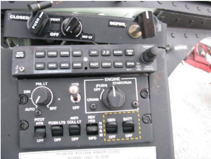
Photo 5 Engine selector switch found in Start/Run position
