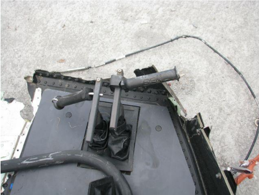
Photo 11 Damage to pilot tail rotor pedals consistent with impact forces
