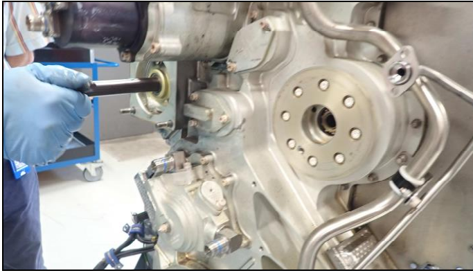
Picture 20 : mechanical continuity check of the accessory gearbox.
