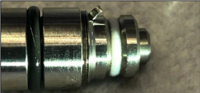
Bearing cage fragment on the electrical magnetic plug #1
