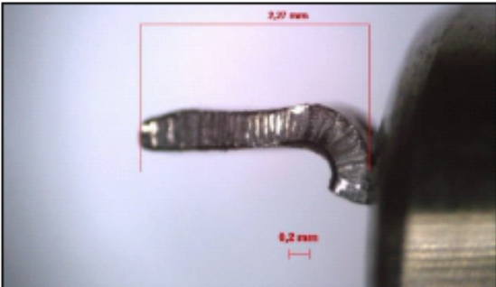
Bearing cage fragment under binocular microscope
